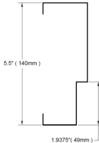
DRAWING PROFILE FOR SINGLE RABBET FRAME DEPTH 5.5"
