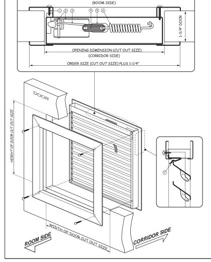
Adjustable Fusible Link Louvers are recommended for use in rooms where ventilation is needed and at the same time isolating the room whenever fire is present. When louver is exposed to heat at 165°F, the fusible link trips and the spring loaded louver blades shut to form an air tight fire and smoke seal.
