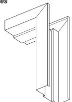
WELDED CORNERS Welded corners are tight fitting to provide a smooth seamless apperance
